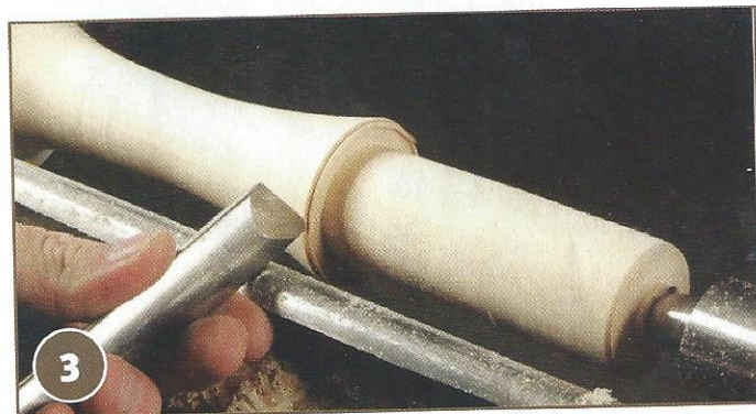
Mount the handle between centres, use the spindle roughing gouge to create the handle form and use a beading/parting tool to create the round tenon. Then, use a skew to create the shoulder
