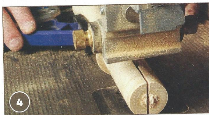
Remove from the lathe and cut the slots for the wedges. The slots should be cut at 90° to each other. Note: the clamp holding the item securely in place
