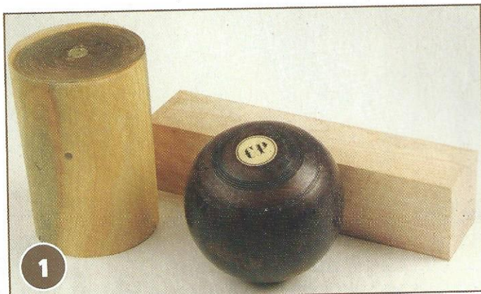
The handle is a pre-dimensioned piece of ash and the mallet head is from lignum – either an old bowling ball or a billet bought from a shop
