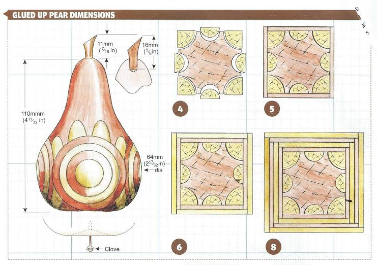
Take a block of sapele measuring 45mm (1<sup>3</sup>/<sub>4</sub>in) x 45mm (1<sup>3</sup>/<sub>4</sub>in) and using a moulding block in a spindle moulder, cut a scotia in two corners
