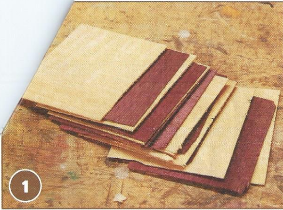
1 Firstly, make your own plywood by gluing stacks of veneer together, as shown here
