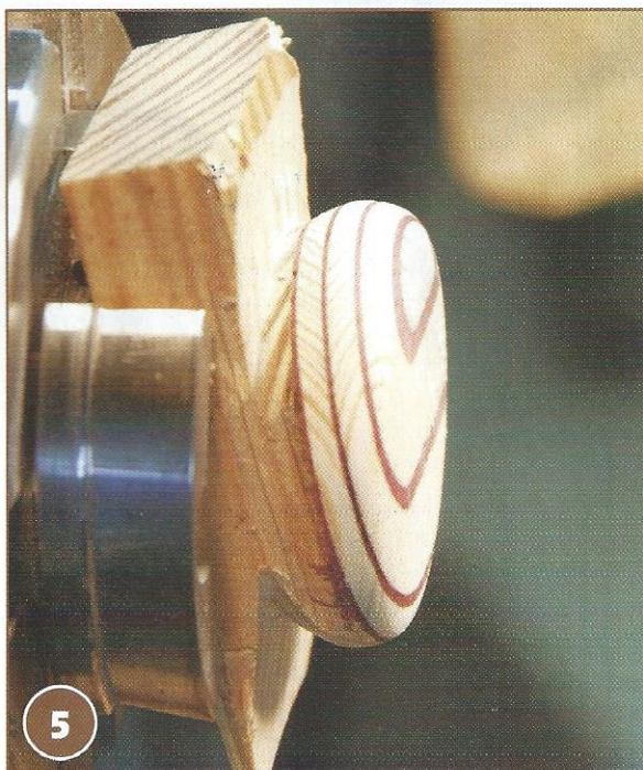
5 When turning, try to make the apex of the outer radius the same as the thin point of the pendant edge
