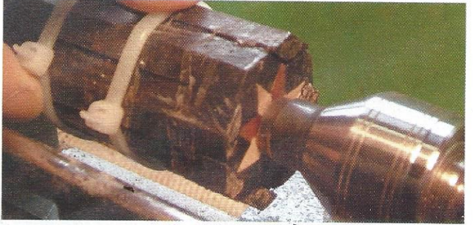
18 The piece will now look like a crude bundle of sticks but do not be dismayed for when cut, surprisingly, the joints will be fine. Set the piece accurately between centres, using a cup centre at the tailstock end and cable ties around the piece to prevent any possible breakout. Rotate the work by hand before switching the lathe on to make sure that nothing catches
