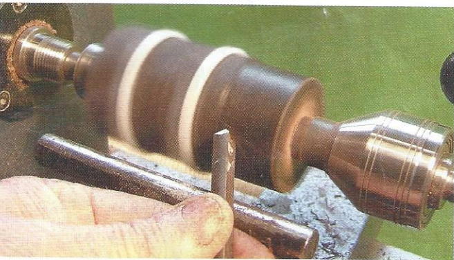
19 Using light cuts, carefully turn the tailstock end of the piece. Wear a face shield – I have never had one of these pieces come apart while turning, but safety first. Note the cable ties around the piece for added security
