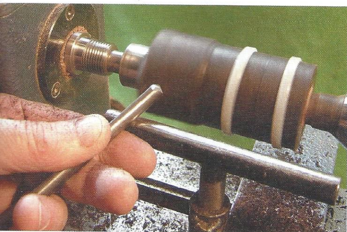
21 Having turned the middle section, the cable tie can be moved on to that turned area and the section closest to the headstock may be completed
