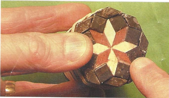
17 Glue the parts together, holding them in place using strong elastic bands
